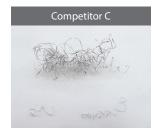
Cutting Conditions : Vc = 400 m/min, ap = 0.3 mm, f = 0.15 mm/rev, Wet, CC \*\* 09T304 Type Workpiece : A6061
