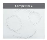
Cutting Conditions : Vc = 400 m/min, ap = 0.5 mm, f = 0.15 mm/rev, Wet, CC \*\* 09T304 Type Workpiece : A6061
