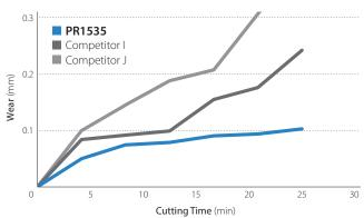
$\begin{array}{l} \mbox{Cutting Conditions: } Vc = 180\mbox{ m/min, } fz = 0.5\mbox{ mm/t, } ap \ x \ ae = 0.3 \times 8\mbox{ mm} \\ \mbox{Cutting Dia. } \emptyset 10, Dry \qquad Workpiece: SUS304 \end{array}$
