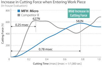
Cutting Conditions: Vc = 120 m/min, fz = 0.6 mm/t, ap = 0.4 mm Cutter Dia. Ø10 mm, Slotting, Dry Workpiece: S50C Cutting Conditions: Vc = 120 m/min, fz = 0.6 mm/t, ap  $\times$  ae = 0.4  $\times$  5 mm Cutter Dia. ø10mm, Dry Workpiece: S50C
