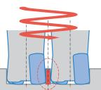
X Under Min. Machining Dia. Center Core Hits Holder Body
