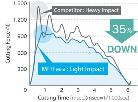
Cutting Conditions : Vc = 150 m/min, ap x ae = 0.5 x 8 mm, fz = 1.0 mm/t, Dry
