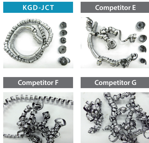
Cutting Conditions : V_c = 150 \text{ m/min} , d = 8 \text{ mm} , f = 0.05 \text{ mm/rev} , Wet Edge Width 4 mm Workpiece Material : SCM415 Grooving
