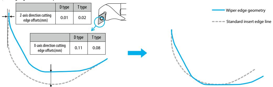
For D type and T type inserts, program corrections are required for ramping and up facing.
