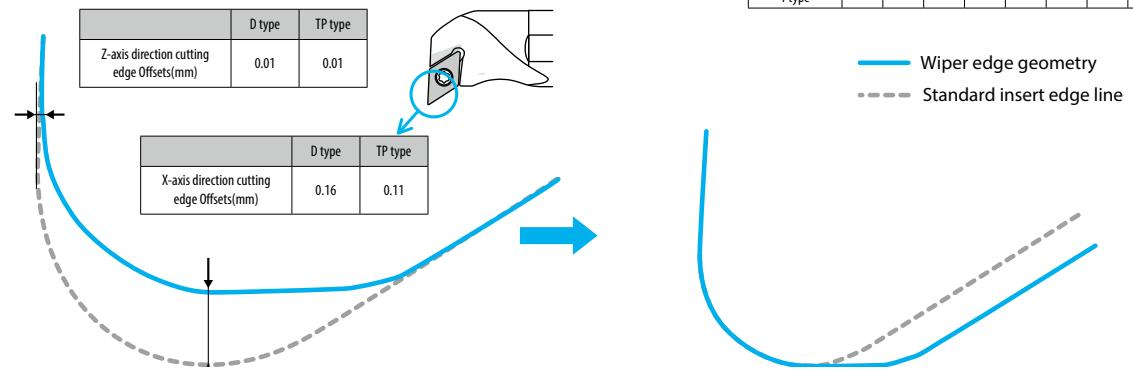
For D type and TP type inserts, program corrections are required for ramping.
