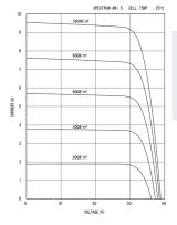
Current-Voltage characteristics of Photovoltaic Module KK280P-3CD3CG at various irradiance levels at Kyocera Corporation laboratory.
